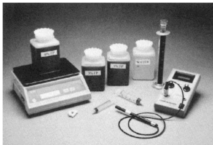
FIGURE B.3(c) Conductivity vs. Concentration — Handheld Conductivity Meter.
